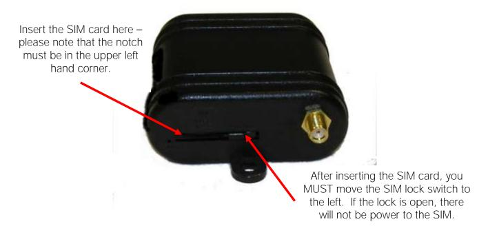
Figure 3 - Inserting a SIM Card in a GSM/GPRS SA-G+ Module
